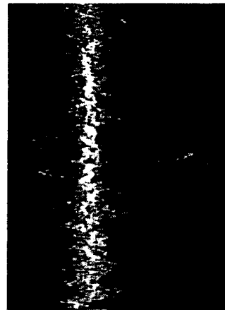
TP FO (Focus out) Vertical : 0.5V/div. Horizontal : 0.5 ms/div. DC, Ground: Center
