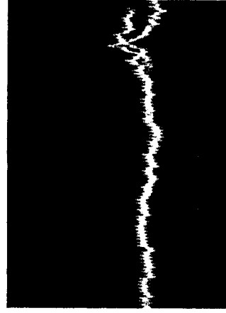
TP SPD (Spindle out) Vertical : 1V/div. Horizontal : 5 ms/div. DC, Ground: Center
